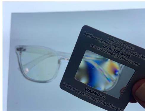
Birefringence depends on wavelength, material thickness and pressure, causing crazy polarization patterns as light passes through them. However, these cool patterns are invisible to the naked eye, so we have to build a simple instrument called a polariscope to reveal them.
